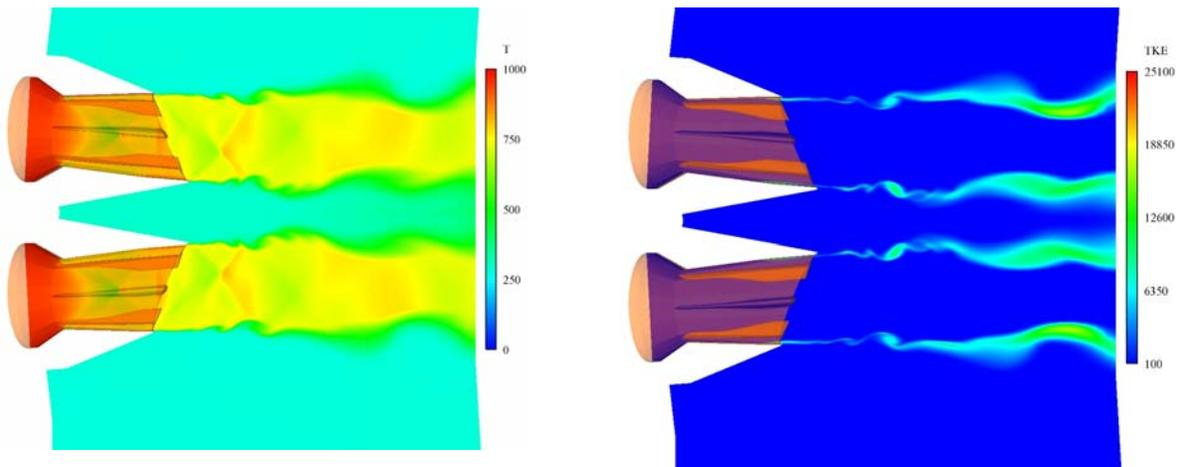
Figure 20. Lobed Nozzle Result of Temperature and TKE at Horizontal Symmetry Plane.
