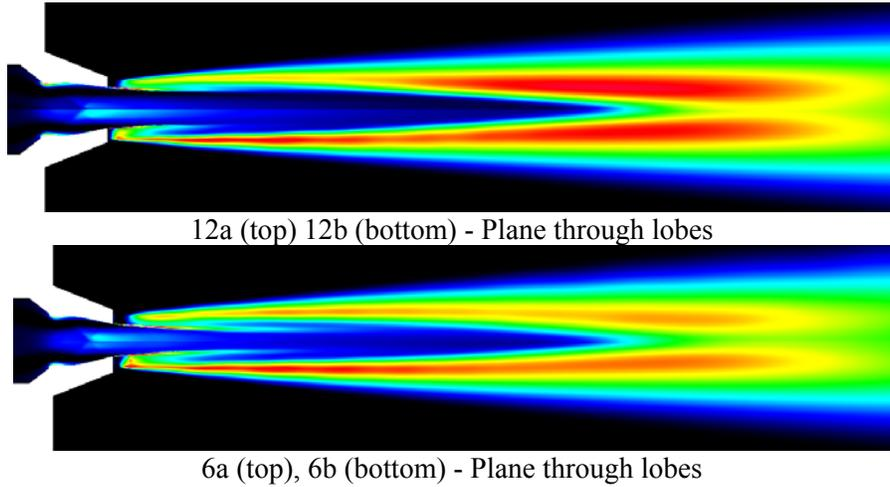
Figure 9. TKE Contours in Symmetry Plane Through Lobes.
