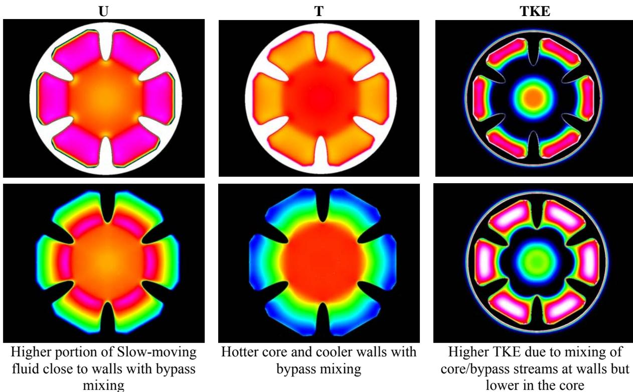
Figure 5. Nozzle Exit Plane Contours with Lobed Noise Reduction Concept Showing Differences Between Subscale Lab Model with Premixed Core/Fan Flow (Upper Fig.) and Real Exhaust (Lower Fig.) with Distributed By-Pass Flow.
