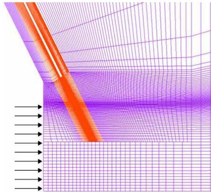
Figure 7. CFD Grid in Plane of Micro-Jet Injector.
