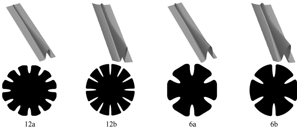
Figure 8. Lobe Configurations for 1/10th Laboratory Model Nozzle.
