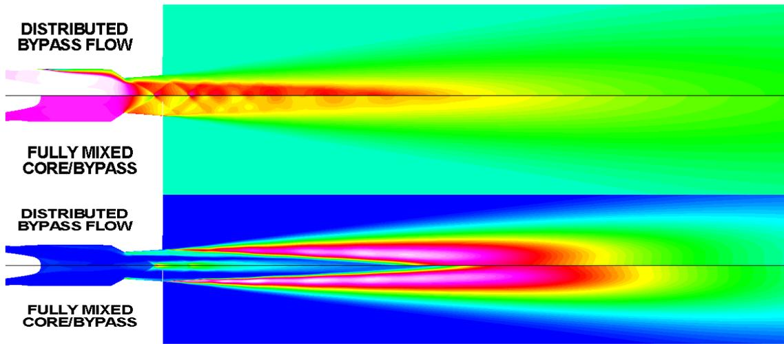
Figure 4. Comparison of Mach number (upper fig.) and TKE contours (lower fig.) for real engine with distributed exhaust and subscale model with premixed core/bypass flow.
