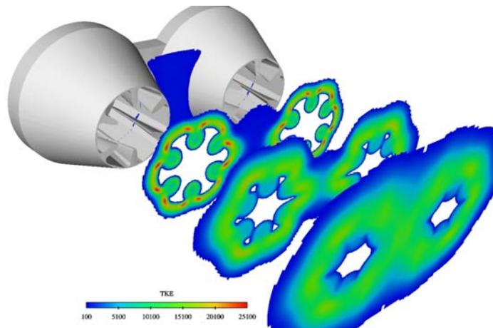
Figure 16. TKE Contours for 6-Lobe Nozzle Dual Plume Calculation.
