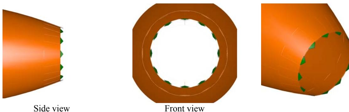
Figure 6. 12 chevrons arranged symmetrically in 30 deg. intervals.
