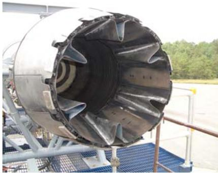
Figure 12. Gas Turbine Engine On Test Stand With Lobes (Corrugated Engine Seals).
