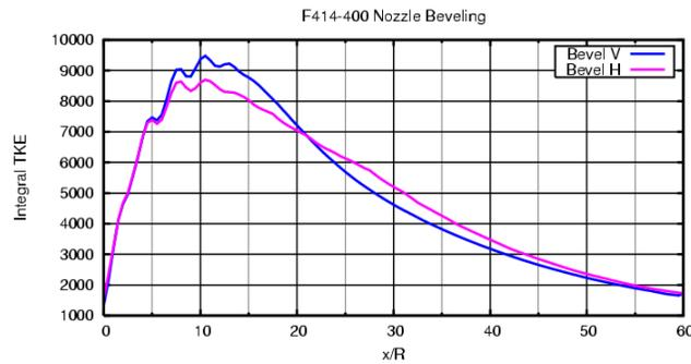
Figure 19. Integral TKE Comparison of Horizontal and Vertical Dual Nozzle, 24 Degree Beveled Configurations.
