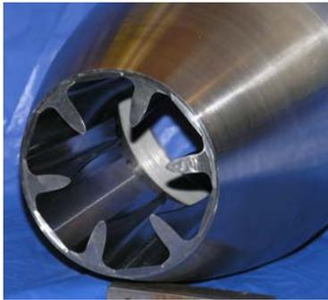
Figure 11. 1/10<sup>th</sup> Scale Model Nozzle with lobes installed.
