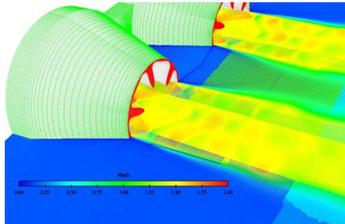
Figure 15. Mach Number Contours Superimposed on Multi-element Unstructured Grid for Dual Nozzle Study with 6 Lobes.
