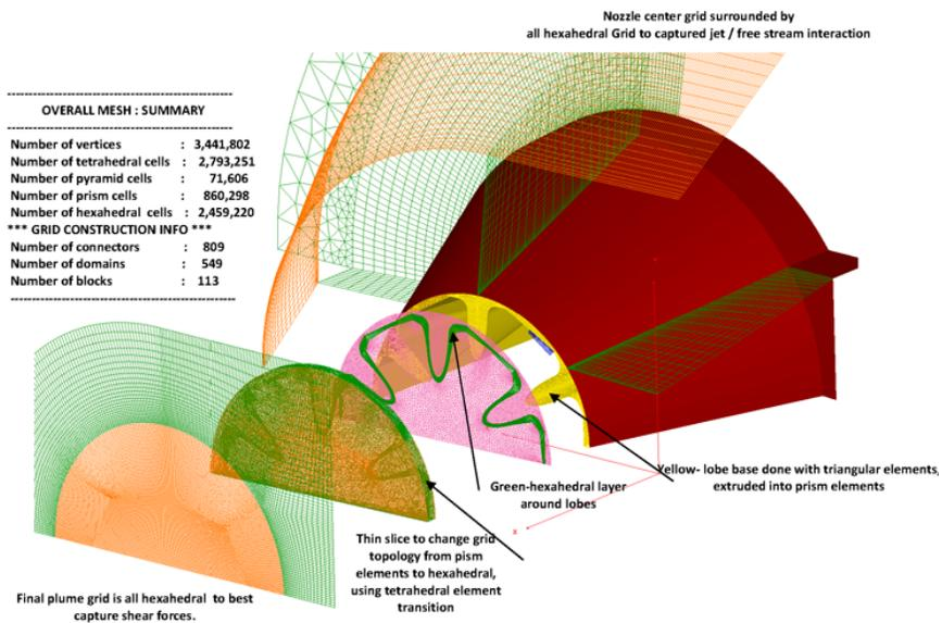
Figure 14. Multi-element Unstructured Grid for Nozzle with 6 Lobes.
