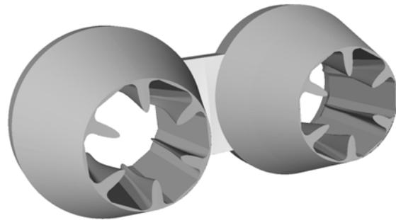
Figure 13. Dual Nozzle Geometry with 6 Lobes
