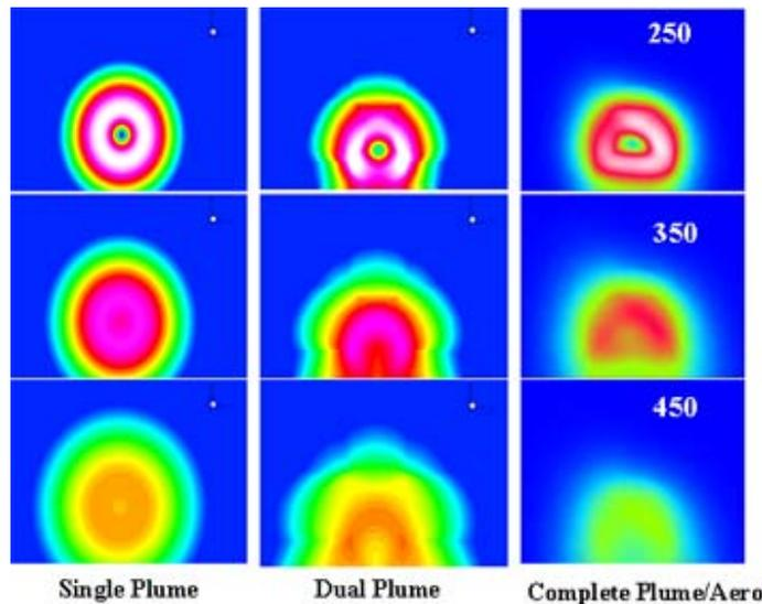
Figure 2. Comparisons of Single & Dual Plume Solutions, and, Solution with Aerodynamic Interactions for Laboratory Configuration with Closely Spaced Nozzles.
