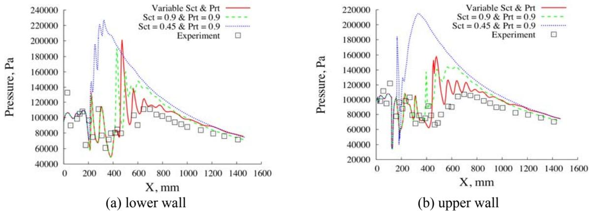
Figure 22. SCHOLAR Combustion Experiment, Wall Pressure Predictions Vs. Data.
