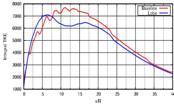
Figure 10. Integral TKE Distribution Along Axial Direction.
