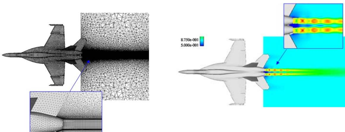
Figure 3. Specialized Multi-Element Grid and Predicted Plume Structure for Dual Nozzle Fighter Aircraft Flowfield.
